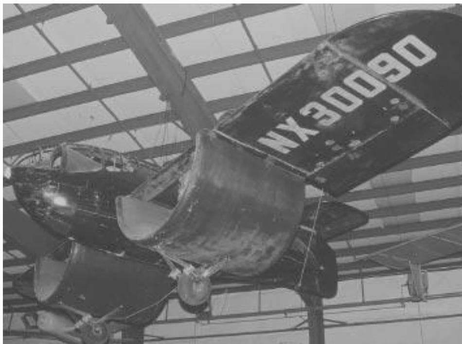
feet were demonstrated. Custer senior calculated that the CCW-2 could lift 11 lbs for every engine horsepower, versus eight for a Piper Cub.
