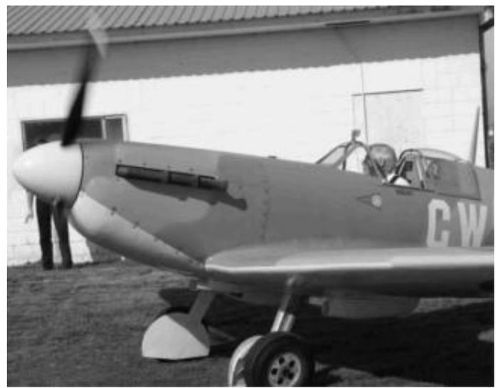
ground adjustable. It is driven through a 4 3/4" wide cog-belt in a 1 to 1 reduction unit also home made. This propeller is a bit too big for the engine so I had to set it in fine pitch to obtain the engine rev's I wanted. I intend to modify the blades a bit to try to improve the performance. However, at 4,000 rev's I was indicating 160 m.p.h.
